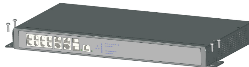
Figure 2-4 Fix the switch on wall
