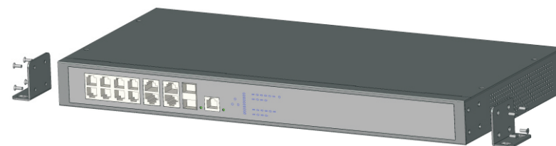
Figure 2-3 Hangers installation diagram
