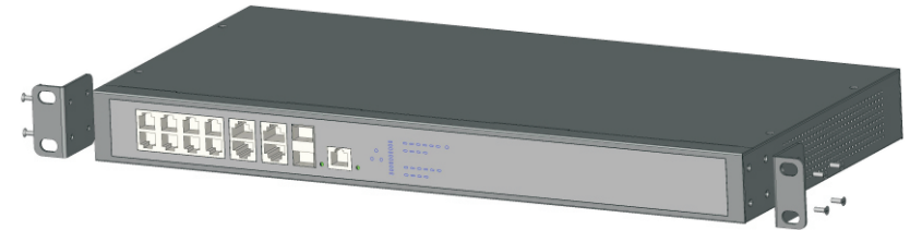
Figure 2-1 Install hangers diagram
