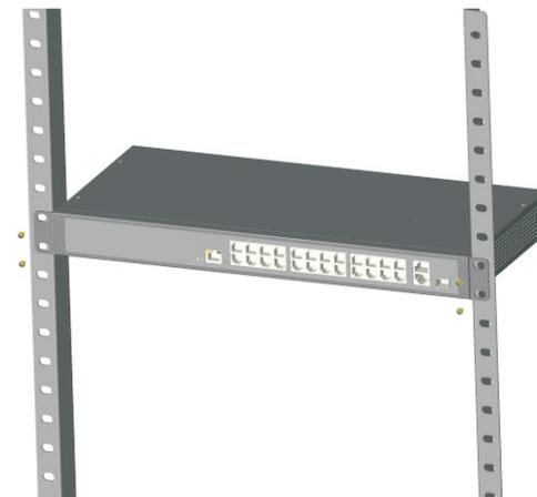
Figure 2-2 Install switch to the rack
