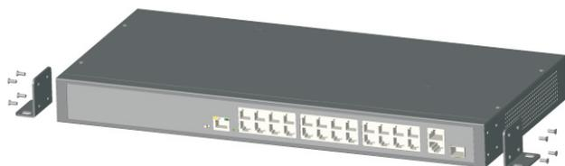
Figure 2-3 Hangers installation diagram
